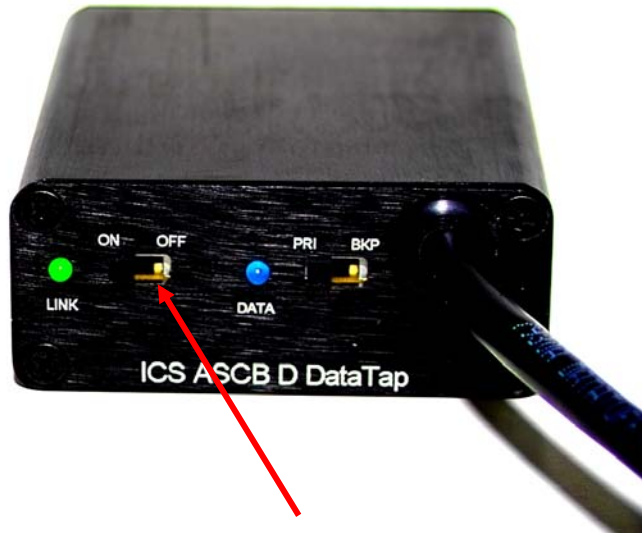
Figure 3-4 FL1400 Bus Interface Adapter Power Switch (Normally Left ON)
